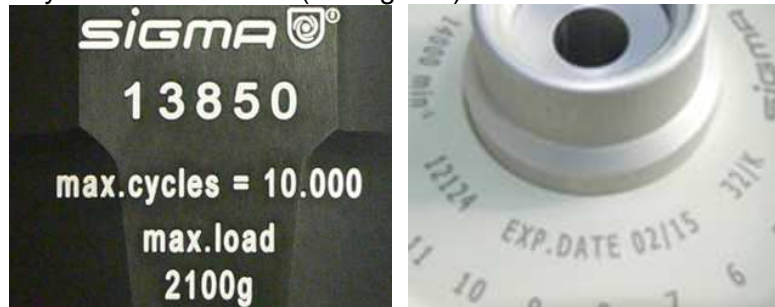
Fig. 5.9: Different service life – engraving on the bucket/rotor
